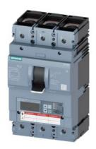
Circuit breaker 3VA6 UL Frame 600 breaking capacity class C 100kA @ 480 V 3-pole, Line protection ETU856, LSI, In=400A overload protection, 100% rated Ir=160A ...400A Short-circuit protection Isd=0.6..10x In, Ii=1.5..12x In N conductor protection optionally with external CT; up to 160% Ground-fault alarm message via EFB300 or COM cable connection on both sides
