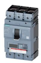
circuit breaker 3VA6 UL frame 600 breaking capacity class C 100kA @ 480 V 3-pole, line protection ETU856, LSI, In=400A overload protection Ir=160A ...400A short-circuit protection Isd=0.6..10x In, Ii=1.5..12x In N conductor protection opt. w. ext. CT; up to 160% ground-fault alarm message via EFB300 or COM cable connection on both sides
