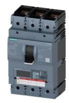
Circuit breaker 3VA6 UL Frame 600 breaking capacity class C 100kA @ 480 V 3pole, Line protection ETU856, LSI, In=400A overload protection, 100% rated Ir=160A ...400A Short-circuit protection Isd=0.6..10x In, Ii=1.5..12x In N conductor protection optionally with external CT; up to 160% Ground-fault alarm message via EFB300 or COM nut keeper kit on both sides
