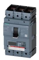
circuit breaker 3VA6 UL frame 600 breaking capacity class C 100kA @ 480 V 3-pole, line protection ETU856, LSI, ln=400A overload protection lr=160A ...400A short-circuit protection lsd=0.6..10x ln, li=1.5..12x ln N conductor protection opt. w. ext. CT; up to 160% ground-fault alarm message via EFB300 or COM nut keeper kit on both sides
