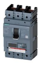
Circuit breaker 3VA6 UL Frame 600 breaking capacity class C 100kA @ 480V 3-pole, Line protection ETU856, LSI, In=400A overload protection, 100% rated Ir=160A...400A Short-circuit protection Isd=0.6...10x In, Ii=1.5..12x In N conductor protection optionally with external CT, up to 160% Ground-fault alarm message via EFB300 or COM without connection
