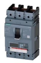
circuit breaker 3VA6 UL frame 600 breaking capacity class C 100kA @ 480V 3pole, line protection ETU856, LSI, In=400A overload protection Ir=160A...400A short-circuit protection Isd=0.6..10x In, Ii=1.5..12x In N conductor protection optionally with external current transformer, up to 160% ground-fault alarm message via EFB300 or COM without connection
