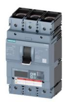
circuit breaker 3VA6 UL frame 600 breaking capacity class C 100kA @ 480 V 3-pole, line protection ETU860, LSIG, In=400A overload protection Ir=160A ...400A short-circuit protection Isd=0.6..10x In, Ii=1.5..12x In N conductor protection opt. w. ext. CT; up to 160% ground-fault protection Ig=0.2... 1 x In, tg=0.05-0.8s cable connection on both sides
