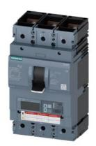
Circuit breaker 3VA6 UL Frame 600 breaking capacity class C 100kA @ 480 V 3-pole, Line protection ETU860, LSIG, In=400A overload protection, 100% rated Ir=160A ...400A Short-circuit protection Isd=0.6..10x In, Ii=1.5..12x In N conductor protection optionally with external CT; up to 160% Ground-fault protection Ig=0.2... 1 x In, tg=0.05-0.8s nut keeper kit on both sides
