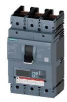
circuit breaker 3VA6 UL frame 600 breaking capacity class C 100kA @ 480V 3pole, line protection ETU860, LSIG, In=400A overload protection Ir=160A...400A short-circuit protection Isd=0.6..10x In, Ii=1.5..12x In N conductor protection optionally with external current transformer, up to 160% ground-fault protection Ig=0.2...1 x In, tg=0.05-0.8s without connection
