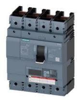
Circuit breaker 3VA6 UL Frame 600 breaking capacity class C 100kA @ 480V 4-pole, Line protection ETU850, LSI, In=400A overload protection, 100% rated Ir=160A...400A Short-circuit protection Isd=0.6..10x In, Ii=1.5..12x In N conductor protection adjustable (OFF, up to 160%) without connection
