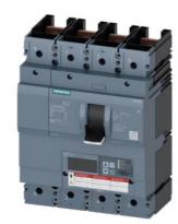
circuit breaker 3VA6 UL frame 600 breaking capacity class C 100kA @ 480V 4pole, line protection ETU850, LSI, In=400A overload protection Ir=160A...400A short-circuit protection Isd=0.6..10x In, Ii=1.5..12x In N conductor protection adjustable (OFF, up to 160%) without connection
