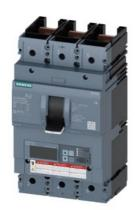
circuit breaker 3VA6 UL frame 600 breaking capacity class C 100kA @ 480V 3-pole, line protection ETU850, LSI, In=400A overload protection Ir=160A...400A short-circuit protection Isd=0.6..10x In, Ii=1.5..12x In N conductor protection optionally with external current transformer, up to 160% without connection
