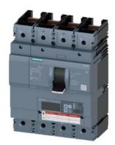
circuit breaker 3VA6 UL frame 600 breaking capacity class C 100kA @ 480V 4-pole, line protection ETU830, LIG, ln=400A overload protection lr=160A...400A short-circuit protection li=1.5...12 x ln ground-fault protection lg=0.2...1 x ln, tg=0.05-0.8s without connection
