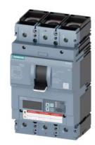
Circuit breaker 3VA6 UL Frame 600 breaking capacity class C 100kA @ 480 V 3pole, Line protection ETU830, LIG, In=400A overload protection, 100% rated Ir=160A ...400A Short-circuit protection Ii=1.5...12 x In Ground-fault protection Ig=0.2... 1 x In, tg=0.05-0.8s cable connection on both sides
