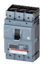
circuit breaker 3VA6 UL frame 600 breaking capacity class C 100kA @ 480 V 3-pole, line protection ETU830, LIG, ln=400A overload protection lr=160A ...400A short-circuit protection li=1.5...12 x ln ground-fault protection lg=0.2... 1 x ln, tg=0.05-0.8s cable connection on both sides
