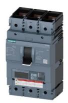
circuit breaker 3VA6 UL frame 600 breaking capacity class C 100kA @ 480 V 3-pole, line protection ETU830, LIG, In=400A overload protection Ir=160A ...400A short-circuit protection li=1.5...12 x ln ground-fault protection lg=0.2... 1 x ln, tg=0.05-0.8s nut keeper kit on both sides
