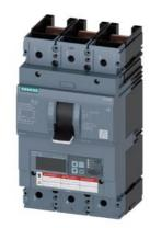
Circuit breaker 3VA6 UL Frame 600 breaking capacity class C 100kA @ 480V 3pole, Line protection ETU830, LIG, In=400A overload protection, 100% rated Ir=160A...400A Short-circuit protection Ii=1.5...12 x In Ground-fault protection Ig=0.2...1 x In, tg=0.05-0.8s without connection
