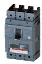
circuit breaker 3VA6 UL frame 600 breaking capacity class C 100kA @ 480V 3-pole, line protection ETU830, LIG, In=400A overload protection Ir=160A...400A short-circuit protection Ii=1.5...12 x In ground-fault protection Ig=0.2...1 x In, tg=0.05-0.8s without connection
