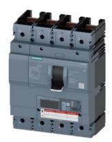
Circuit breaker 3VA6 UL Frame 600 breaking capacity class C 100kA @ 480V 4-pole, Line protection ETU820, LI, In=400A overload protection, 100% rated Ir=160A...400A Short-circuit protection Ii=1.5...12 x In without connection
