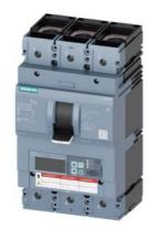
circuit breaker 3VA6 UL frame 600 breaking capacity class C 100kA @ 480 V 3-pole, line protection ETU820, LI, In=400A overload protection Ir=160A ...400A short-circuit protection li=1.5...12 x In cable connection on both sides
