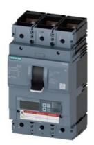
circuit breaker 3VA6 UL frame 600 breaking capacity class C 100kA @ 480 V 3-pole, line protection ETU820, LI, In=400A overload protection Ir=160A ...400A short-circuit protection Ii=1.5...12 x In nut keeper kit on both sides
