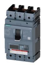
Circuit breaker 3VA6 UL Frame 600 breaking capacity class C 100kA @ 480V 3-pole, Line protection ETU820, LI, In=400A overload protection, 100% rated Ir=160A...400A Short-circuit protection li=1.5...12 x In without connection
