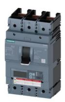
circuit breaker 3VA6 UL frame 600 breaking capacity class C 100kA @ 480V 3-pole, line protection ETU820, LI, In=400A overload protection Ir=160A...400A short-circuit protection Ii=1.5...12 x In without connection
