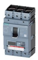
Circuit breaker 3VA6 UL Frame 600 breaking capacity class C 100kA @ 480 V 3-pole, Line protection ETU556, LSI, In=400A overload protection, 100% rated Ir=160A ...400A Short-circuit protection Isd=0.6..10x In, Ii=1.5..12x In N conductor protection optionally with external CT; up to 160% Ground-fault alarm message via EFB300 or COM cable connection on both sides
