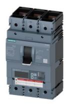
Circuit breaker 3VA6 UL Frame 600 breaking capacity class C 100kA @ 480 V 3-pole, Line protection ETU556, LSI, In=400A overload protection, 100% rated Ir=160A ...400A Short-circuit protection Isd=0.6..10x In, Ii=1.5..12x In N conductor protection optionally with external CT; up to 160% Ground-fault alarm message via EFB300 or COM nut keeper kit on both sides
