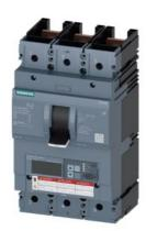
circuit breaker 3VA6 UL frame 600 breaking capacity class C 100kA @ 480V 3-pole, line protection ETU556, LSI, In=400A overload protection Ir=160A...400A short-circuit protection Isd=0.6..10x In, Ii=1.5..12x In N conductor protection optionally with external current transformer, up to 160% ground-fault alarm message via EFB300 or COM without connection
