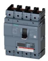
Circuit breaker 3VA6 UL Frame 600 breaking capacity class C 100kA @ 480V 4-pole, Line protection ETU560, LSIG, In=400A overload protection, 100% rated Ir=160A...400A Short-circuit protection Isd=0.6..10x In, Ii=1.5..12x In N conductor protection adjustable (OFF, up to 160%) Ground-fault protection Ig=0.2...1 x In=tg=0.05-0.8s without connection
