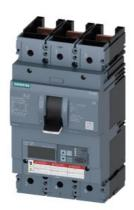
Circuit breaker 3VA6 UL Frame 600 breaking capacity class C 100kA @ 480V 3-pole, Line protection ETU560, LSIG, In=400A overload protection, 100% rated Ir=160A...400A Short-circuit protection Isd=0.6..10x In, Ii=1.5..12x In N conductor protection optionally with external CT, up to 160% Ground-fault protection Ig=0.2...1 x In, tg=0.05-0.8s without connection
