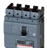
circuit breaker 3VA6 UL frame 600 breaking capacity class C 100kA @ 480V 4-pole, line protection ETU550, LSI, In=400A overload protection Ir=160A...400A short-circuit protection Isd=0.6..10x In, Ii=1.5..12x In N conductor protection adjustable (OFF, up to 150%) without connection
