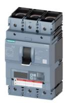
Circuit breaker 3VA6 UL Frame 600 breaking capacity class C 100kA @ 480 V 3-pole, Line protection ETU550, LSI, In=400A overload protection, 100% rated Ir=160A ...400A Short-circuit protection Isd=0.6..10x In, Ii=1.5..12x In N conductor protection optionally with external CT; up to 160% cable connection on both sides
