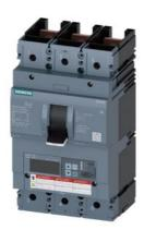
Circuit breaker 3VA6 UL Frame 600 breaking capacity class C 100kA @ 480V 3-pole, Line protection ETU550, LSI, In=400A overload protection, 100% rated Ir=160A...400A Short-circuit protection Isd=0.6..10x In, Ii=1.5..12x In N conductor protection optionally with external CT, up to 160% without connection
