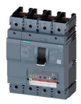
Circuit breaker 3VA6 UL Frame 600 breaking capacity class C 100kA @ 480V 4-pole, Line protection ETU350, LSI, In=400A overload protection, 100% rated Ir=160A...400A Short-circuit protection Isd=1.5...10 x Ir, Ii=12 x In N conductor protection adjustable (OFF, 50%, 100%) without connection
