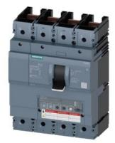
circuit breaker 3VA6 UL frame 600 breaking capacity class C 100kA @ 480V 4-pole, line protection ETU350, LSI, In=400A overload protection Ir=160A...400A short-circuit protection Isd=1.5...10 x Ir, Ii=12 x In N conductor protection adjustable (OFF, 50%, 100%) without connection
