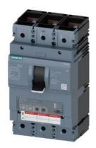
Circuit breaker 3VA6 UL Frame 600 breaking capacity class C 100kA @ 480 V 3-pole, Line protection ETU350, LSI, In=400A overload protection, 100% rated Ir=160A ...400A Short-circuit protection Isd=1.5... 10 x Ir, Ii=12 x In nut keeper kit on both sides
