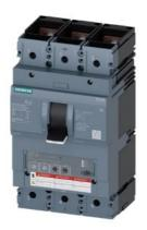
circuit breaker 3VA6 UL frame 600 breaking capacity class C 100kA @ 480 V 3-pole, line protection ETU350, LSI, In=400A overload protection Ir=160A ...400A short-circuit protection Isd=1.5... 10 x Ir, Ii=12 x In nut keeper kit on both sides
