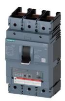
Circuit breaker 3VA6 UL Frame 600 breaking capacity class C 100kA @ 480V 3-pole, Line protection ETU350, LSI, In=400A overload protection, 100% rated Ir=160A...400A Short-circuit protection Isd=1.5...10 x Ir, Ii=12 x In without connection
