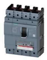
Circuit breaker 3VA6 UL Frame 600 breaking capacity class C 100kA @ 480V 4-pole, Line protection ETU330, LIG, In=400A overload protection, 100% rated Ir=160A...400A Short-circuit protection Ii=1.5...12 x In N conductor protection adjustable (OFF, 50%, 100%) Ground-fault protection Ig=0.2...1 x In= tg=0.1/0.3s without connection
