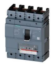
circuit breaker 3VA6 UL frame 600 breaking capacity class C 100kA @ 480V 4-pole, line protection ETU330, LIG, In=400A overload protection Ir=160A...400A short-circuit protection li=1.5...12 x In N conductor protection adjustable (OFF, 50%, 100%) ground-fault protection Ig=0.2...1 x In= tg=0.1/0.3s without connection
