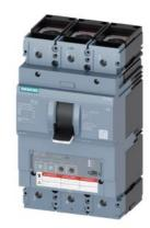
circuit breaker 3VA6 UL frame 600 breaking capacity class C 100kA @ 480 V 3-pole, line protection ETU330, LIG, In=400A overload protection Ir=160A ...400A short-circuit protection li=1.5...12 x In ground-fault protection Ig=0.2... 1 x In, tg=0.1/0.3s cable connection on both sides
