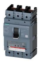
Circuit breaker 3VA6 UL Frame 600 breaking capacity class C 100kA @ 480V 3-pole, Line protection ETU330, LIG, ln=400A overload protection, 100% rated lr=160A...400A Short-circuit protection li=1.5...12 x ln Ground-fault protection lg=0.2...1 x ln, tg=0.1/0.3s without connection
