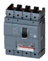
Circuit breaker 3VA6 UL Frame 600 breaking capacity class C 100kA @ 480V 4-pole, Line protection ETU320, LI, In=400A overload protection, 100% rated Ir=160A...400A Short-circuit protection Ii=1.5...12 x In N conductor protection adjustable (OFF, 50%, 100%) without connection
