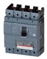
circuit breaker 3VA6 UL frame 600 breaking capacity class C 100kA @ 480V 4-pole, line protection ETU320, LI, ln=400A overload protection lr=160A...400A short-circuit protection li=1.5...12 x ln N conductor protection adjustable (OFF, 50%, 100%) without connection
