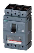
circuit breaker 3VA6 UL frame 600 breaking capacity class C 100kA @ 480 V 3-pole, line protection ETU320, LI, In=400A overload protection Ir=160A ...400A short-circuit protection li=1.5...12 x In nut keeper kit on both sides
