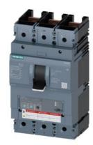
Circuit breaker 3VA6 UL Frame 600 breaking capacity class C 100kA @ 480V 3-pole, Line protection ETU320, LI, In=400A overload protection, 100% rated Ir=160A...400A Short-circuit protection li=1.5...12 x In without connection
