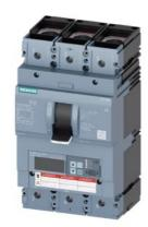
Circuit breaker 3VA6 UL Frame 600 breaking capacity class H 65kA @ 480 V 3pole, Line protection ETU856, LSI, In=400A overload protection, 100% rated Ir=160A ...400A Short-circuit protection Isd=0.6..10x In, Ii=1.5..12x In N conductor protection optionally with external CT; up to 160% Ground-fault alarm message via EFB300 or COM cable connection on both sides
