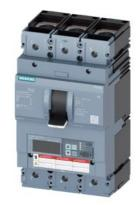
circuit breaker 3VA6 UL frame 600 breaking capacity class H 65kA @ 480 V 3pole, line protection ETU856, LSI, In=400A overload protection Ir=160A ...400A short-circuit protection Isd=0.6..10x In, Ii=1.5..12x In N conductor protection opt. w. ext. CT; up to 160% ground-fault alarm message via EFB300 or COM cable connection on both sides
