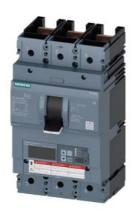
Circuit breaker 3VA6 UL Frame 600 breaking capacity class H 65kA @ 480V 3-pole, Line protection ETU856, LSI, In=400A overload protection, 100% rated Ir=160A...400A Short-circuit protection Isd=0.6..10x In, Ii=1.5..12x In N conductor protection optionally with external CT, up to 160% Ground-fault alarm message via EFB300 or COM without connection
