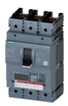
circuit breaker 3VA6 UL frame 600 breaking capacity class H 65kA @ 480V 3-pole, line protection ETU856, LSI, In=400A overload protection Ir=160A...400A short-circuit protection Isd=0.6..10x In, Ii=1.5..12x In N conductor protection optionally with external current transformer, up to 160% ground-fault alarm message via EFB300 or COM without connection
