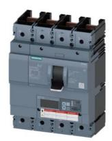
Circuit breaker 3VA6 UL Frame 600 breaking capacity class H 65kA @ 480V 4-pole, Line protection ETU860, LSIG, In=400A overload protection, 100% rated Ir=160A...400A Short-circuit protection Isd=0.6..10x In, Ii=1.5..12x In N conductor protection adjustable (OFF, up to 160%) Ground-fault protection Ig=0.2...1 x In=tg=0.05-0.8s without connection
