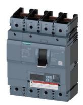
circuit breaker 3VA6 UL frame 600 breaking capacity class H 65kA @ 480V 4-pole, line protection ETU860, LSIG, In=400A overload protection Ir=160A...400A short-circuit protection Isd=0.6..10x In, Ii=1.5..12x In N conductor protection adjustable (OFF, up to 160%) ground-fault protection Ig=0.2...1 x In= tg=0.05-0.8s without connection
